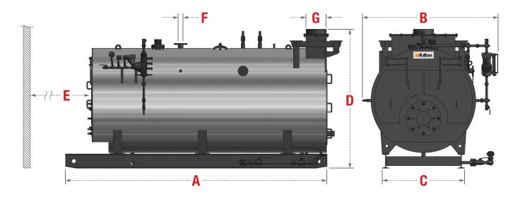
STEAM MODELS: 2,070 - 16,387 lbs/h Output F&A 212°F ASME Section IV & I Designs to 300psi HOT WATER MODELS: 2 MM - 15.9 MM Btu/hr ASME Section I & IV designs **NOTE:** Specifications and dimensions are approximate and for reference only. Fulton practices continuous product improvement and reserves the right to change specifications and/or dimensions without notice.
